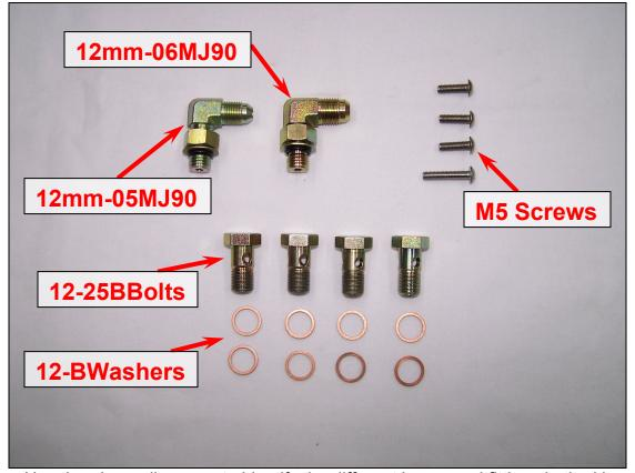
Use the above diagrams to identify the different hoses and fittings in the kit
