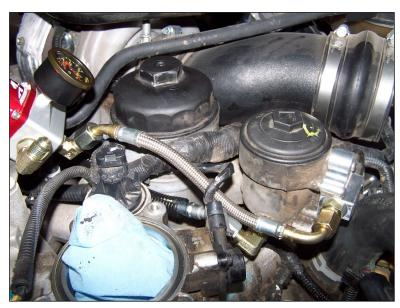
NOTE: In the next steps we will be working on the fittings on the rear of the cylinder heads. Access to these fittings is tight and can be difficult. We've supplied a long handled 6mm allen wrench to help, but because the fittings don't necessarily orient themselves ideally when installed, you may need to modify our tool (shorten or bend the handle) or use one of your own. These fittings are tight, but once broken free they can usually be removed quite easily by hand.
